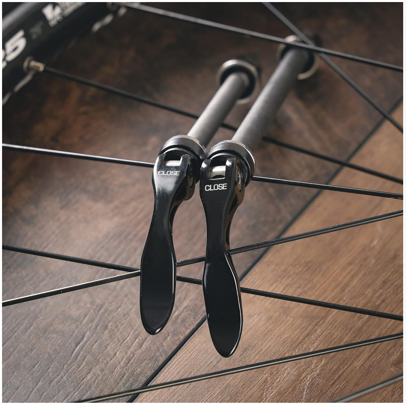
Figure 3: Quick release skewers properly installed through a bicycle wheel hub.
