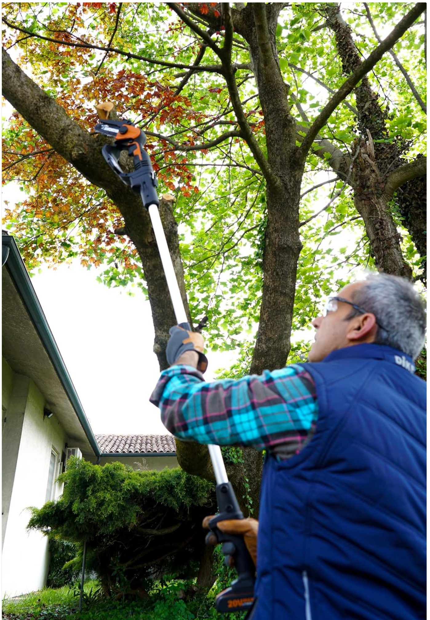
Image 2: A user operating the WORX extension pole with a mini chainsaw to prune a high tree branch.
