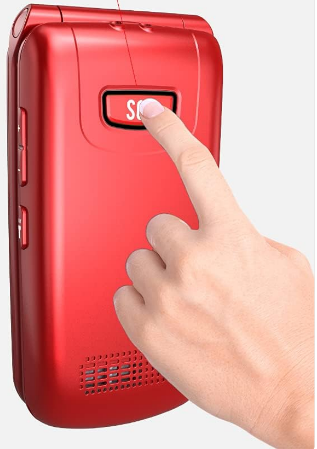
Figure 5.1: The SOS emergency call feature allows users to quickly reach up to five pre-selected family members or emergency contacts by pressing the dedicated SOS button.
