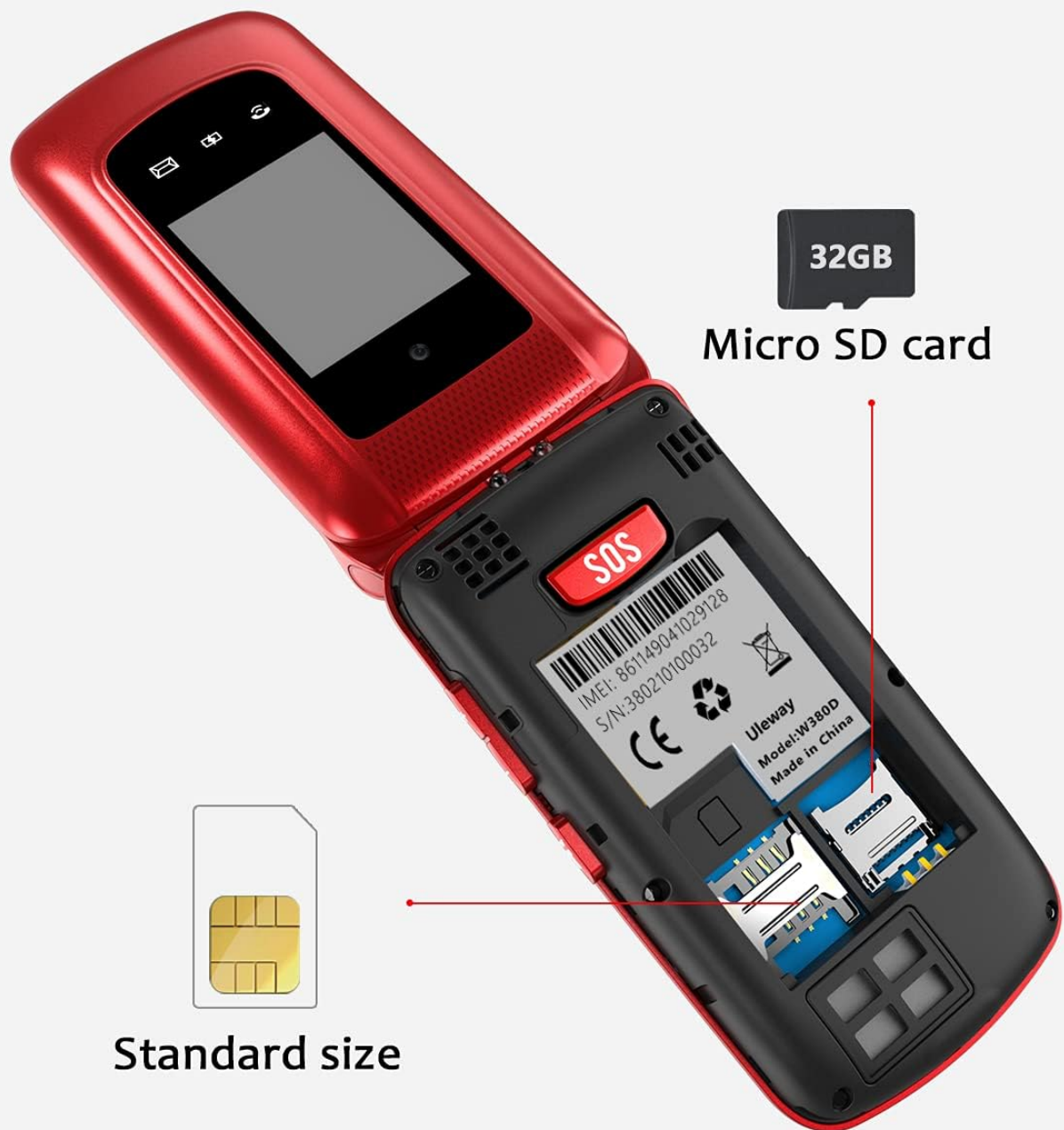
Figure 4.1: Internal view of the phone, illustrating the placement of the standard-sized SIM card and the Micro SD card for memory expansion.
