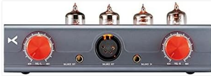
Figure 1: Front view of the XDUOO MT-604 amplifier, showing the dual volume controls, 4.4mm and XLR balanced inputs, and 4.4mm and 4-pin XLR balanced outputs.
