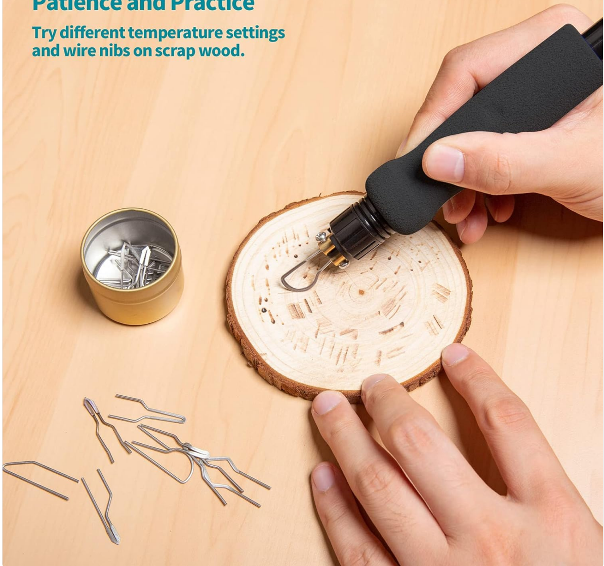
Image 5.2: A user practicing wood burning on a small circular wood slice, demonstrating the importance of trying different temperature settings and wire nibs on scrap wood to achieve desired results.
