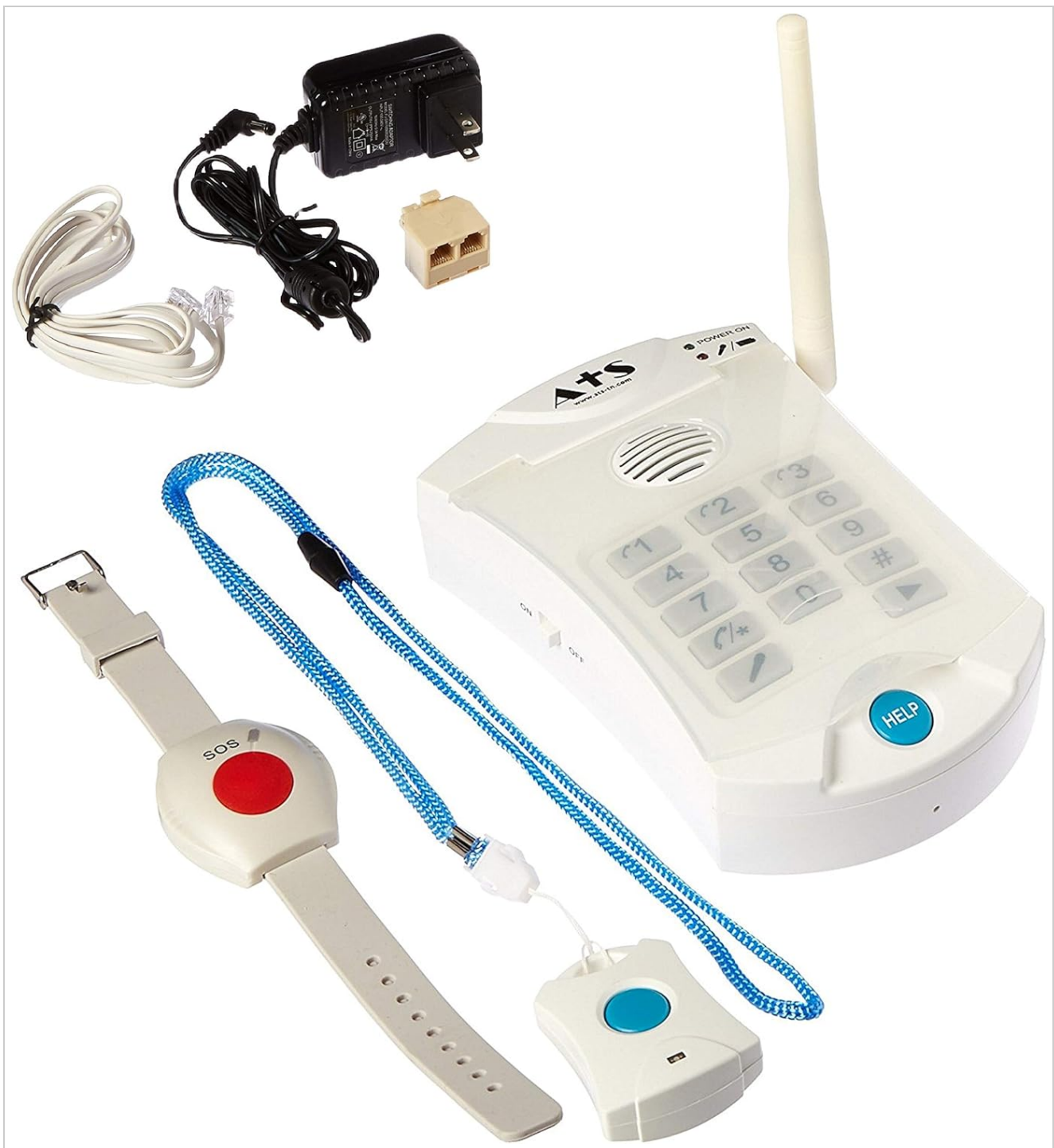
Image 4.2: The necklace panic button, designed for easy access and activation.
