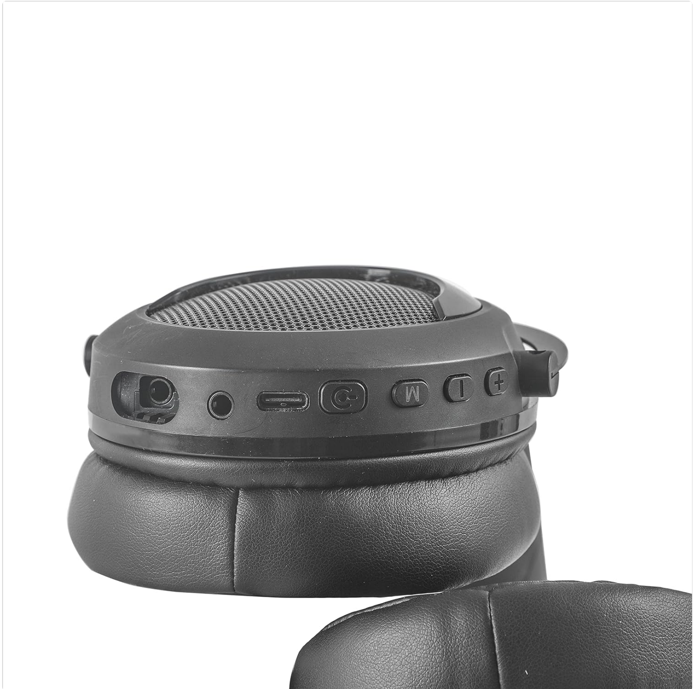
Image 4.1: Close-up view of the control panel on the left ear cup, showing the 3.5mm jack, USB-C charging port, power button, mode button, and volume controls.
