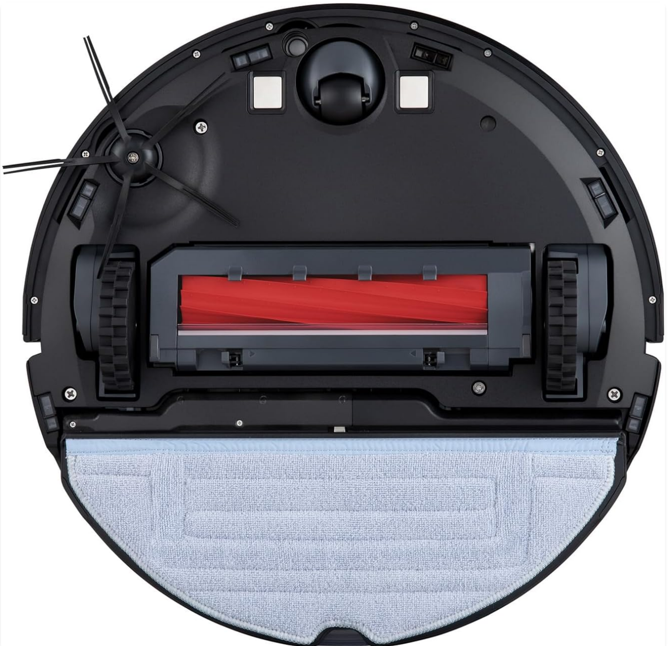
Figure 5.1: Location of the main brush on the underside of the robot vacuum for maintenance.
