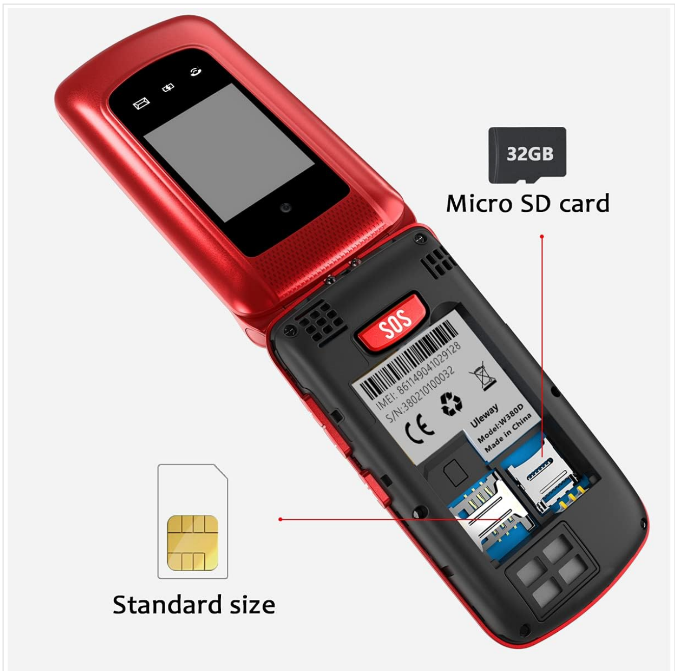
Image: Illustration of SIM card and Micro SD card insertion into the phone's internal slots.
