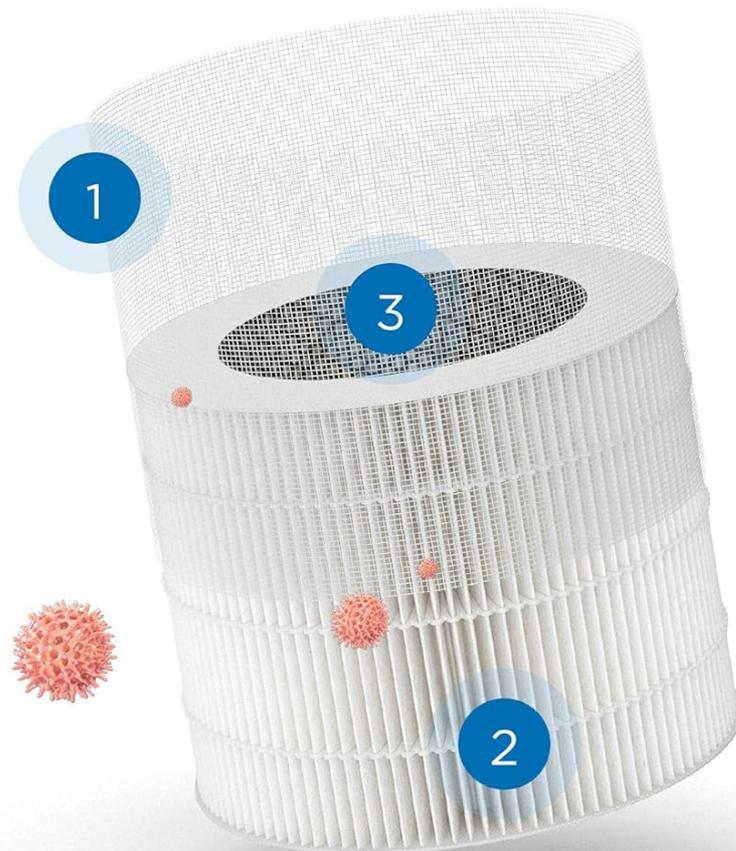
Image: A detailed diagram showing the 3-stage filter: 1) Pre-filter for large particles, 2) H13 HEPA filter for 99.9% of particles down to 0.1 microns, and 3) Activated carbon filter for odors.
