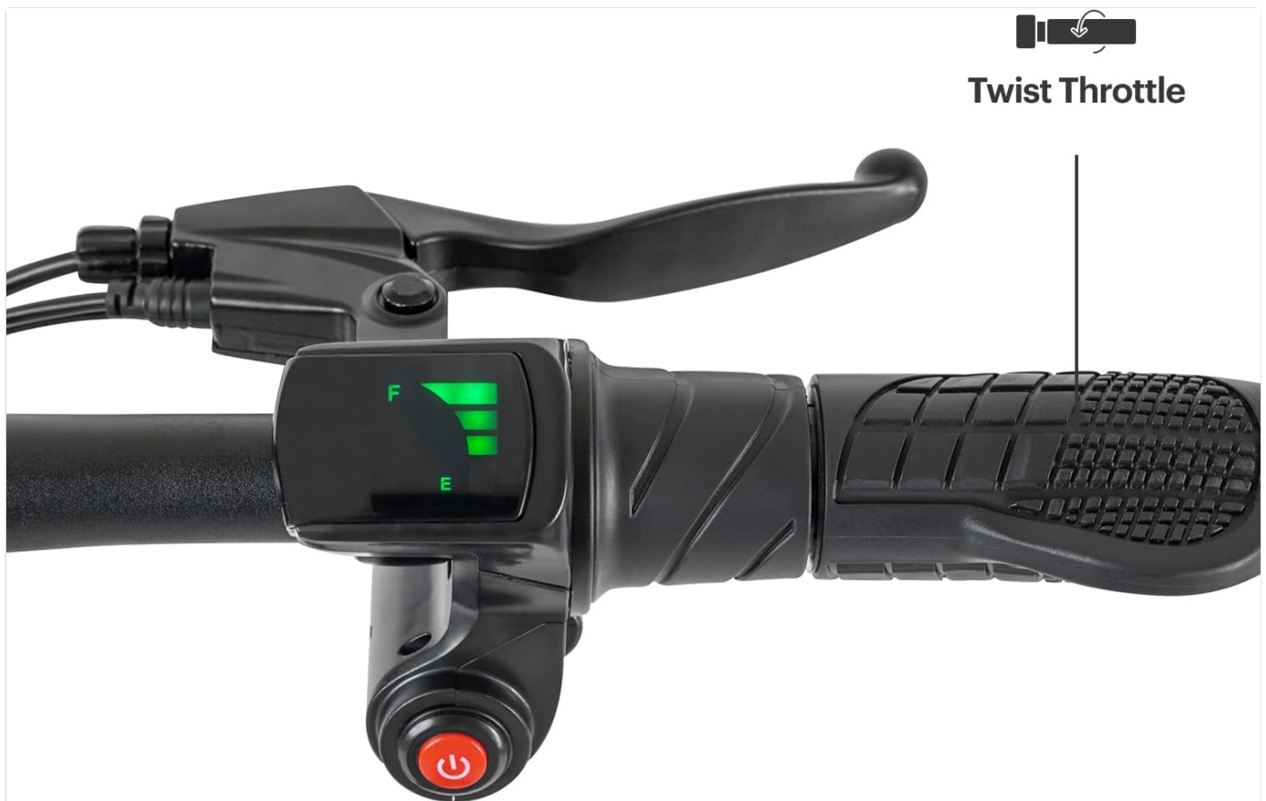
Image: A detailed view of the handlebar, showing the twist throttle and the LCD display which indicates battery level and speed.
