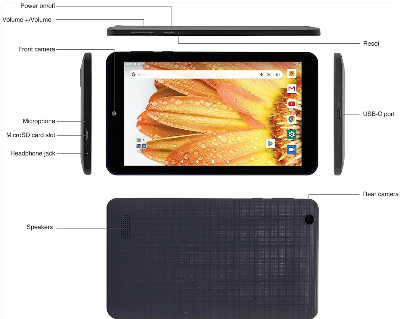
Figure 1: Tablet Components Diagram. This image displays the Venturer Voyager 7 Inch Tablet from multiple angles, highlighting key features such as the Power on/off button, Volume +/Volume - buttons, Front camera, Reset button, USB-C port, Microphone, MicroSD card slot, Headphone jack, Rear camera, and Speakers.
