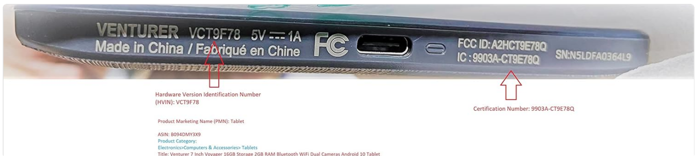
Figure 5: Model and Certification Details. This image shows the back of the Venturer Voyager 7 Inch Tablet, displaying the model number (VCT9F78), power input (5V === 1A), FCC ID (2IHCT9E78Q), and IC (3903A-CT9E78Q), along with the "Made in China" label.
