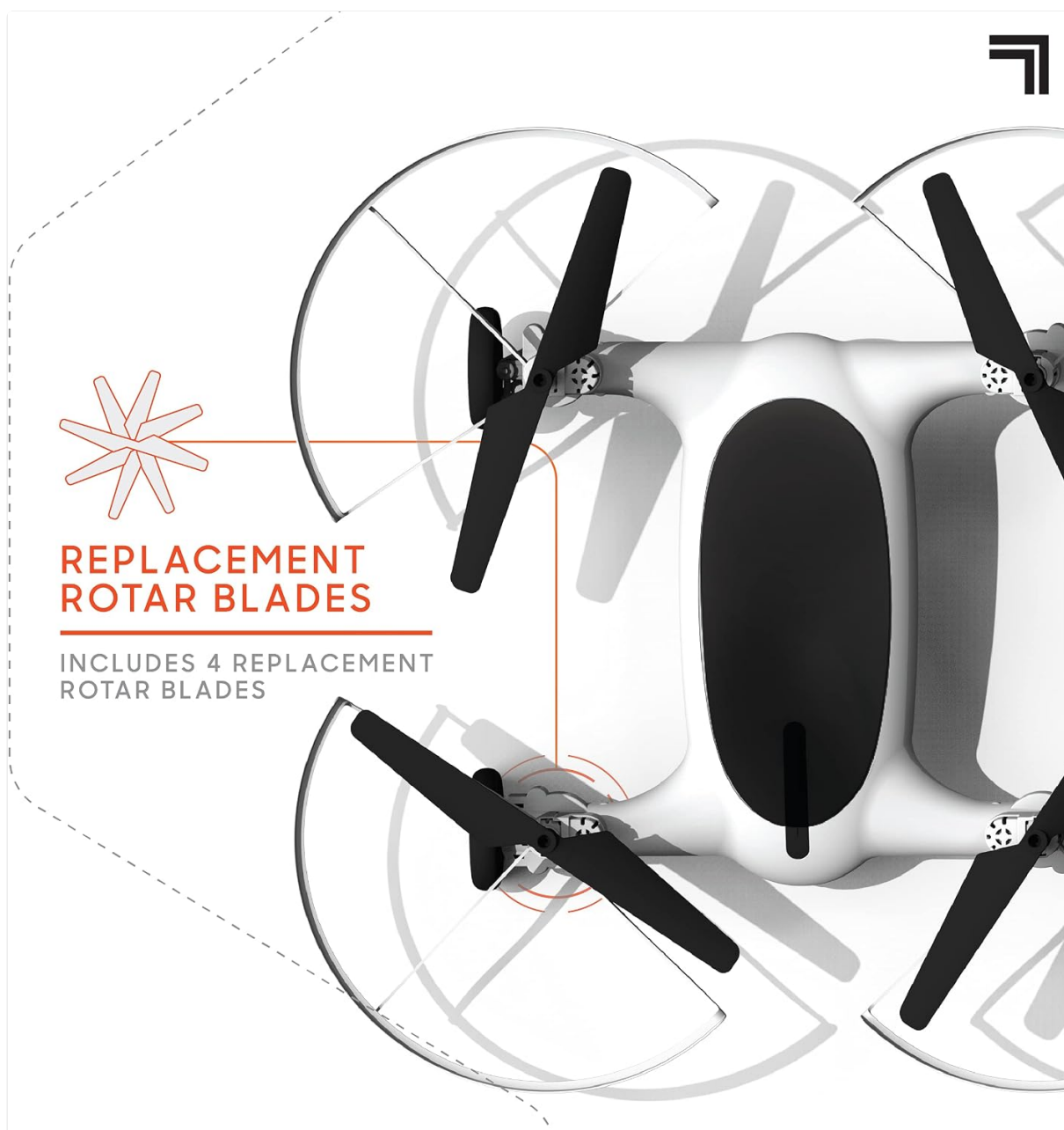
Image: A close-up view illustrating the replacement rotor blades and their attachment points on the drone.
