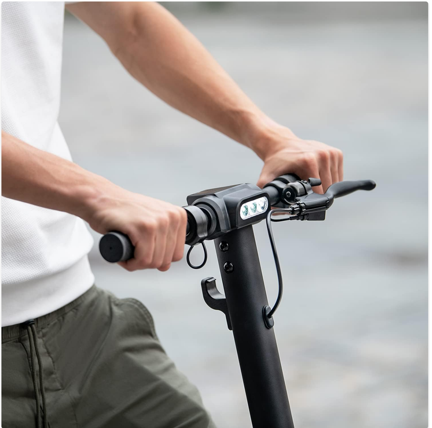
Figure 7: LCD display showing speed, battery, and mileage.
