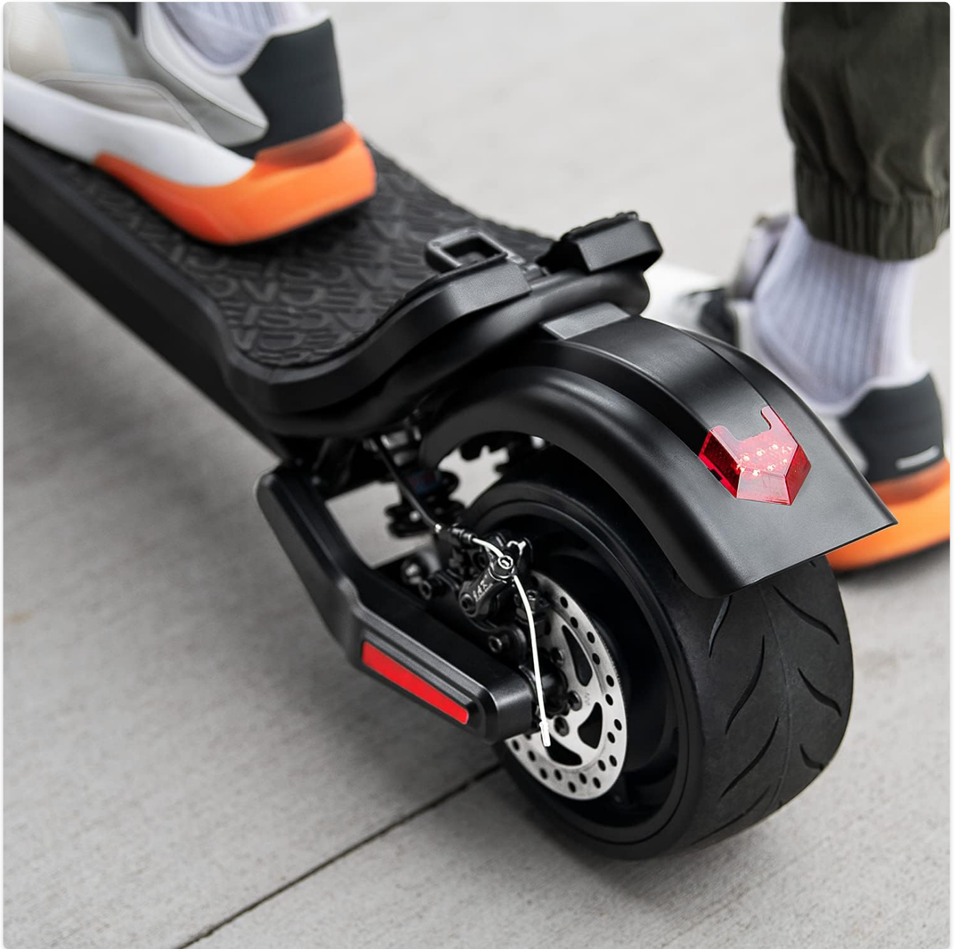
Figure 9: The rear disc brake system for effective stopping.
