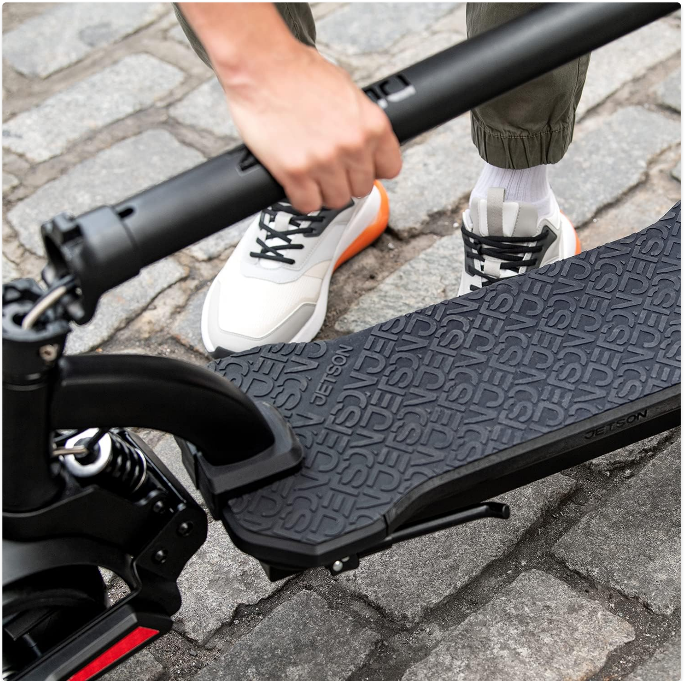
Figure 5: Detail of the easy folding mechanism.
