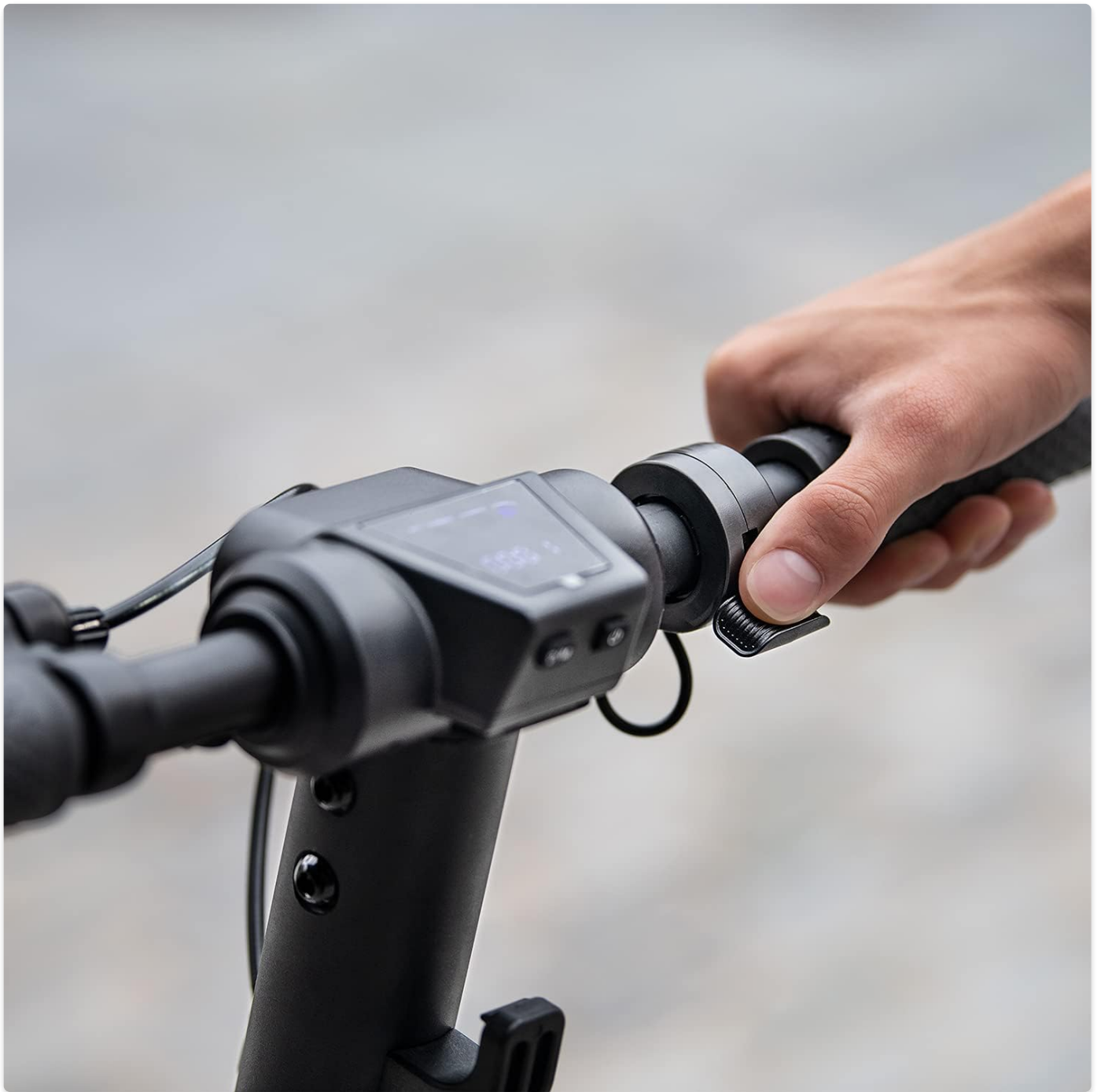
Figure 8: The thumb throttle for acceleration.
