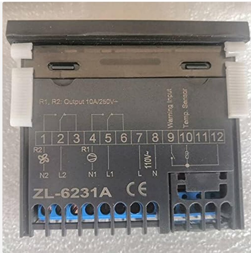
Figure 5.1: Rear view of the ZL-6231A Incubator Controller, detailing the wiring terminals (1-12) and the integrated schematic diagram for electrical connections.
