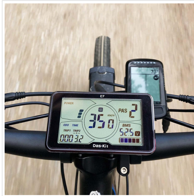
Image 5.1: An e-bike display showing a speed of 35 km/h, indicating the tuning chip's effect on the maximum assisted speed.
