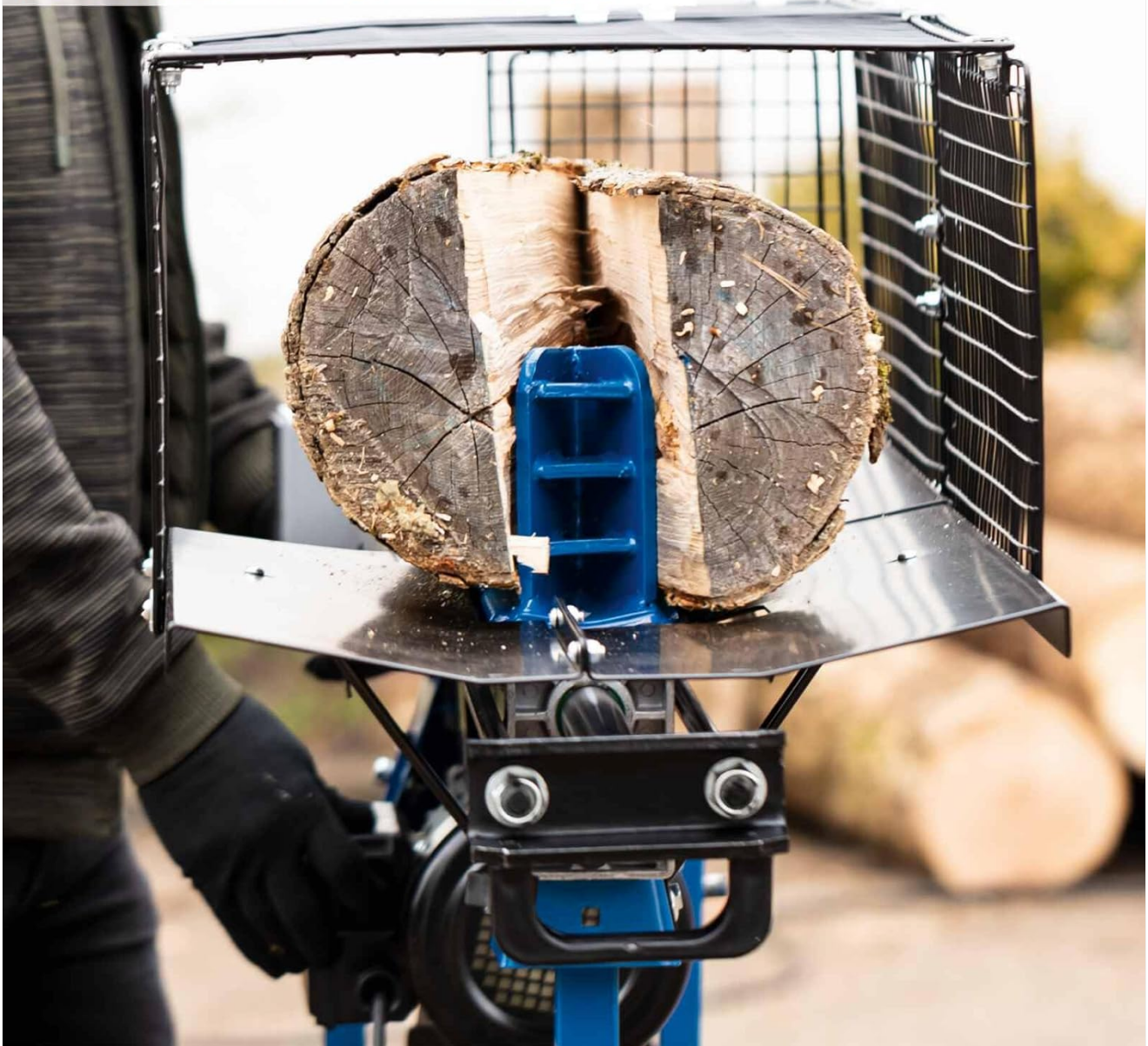
Figure 3.2: A log being processed by the HL760LS, demonstrating its splitting action.
