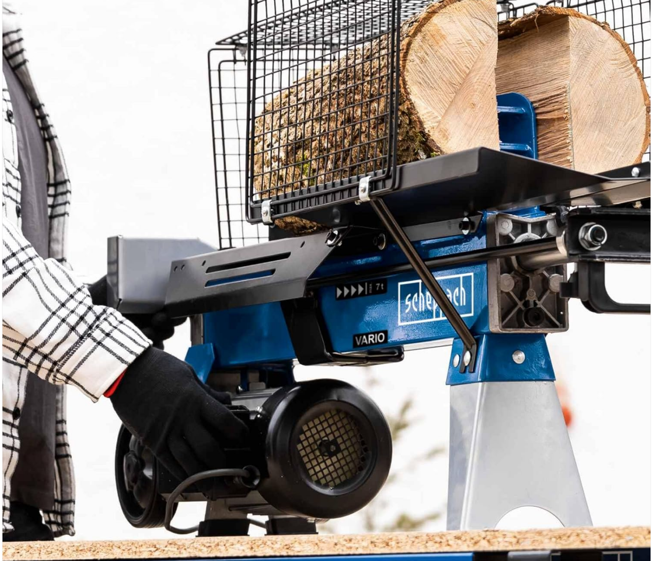
Figure 3.3: Proper two-hand operation of the log splitter for safety.
