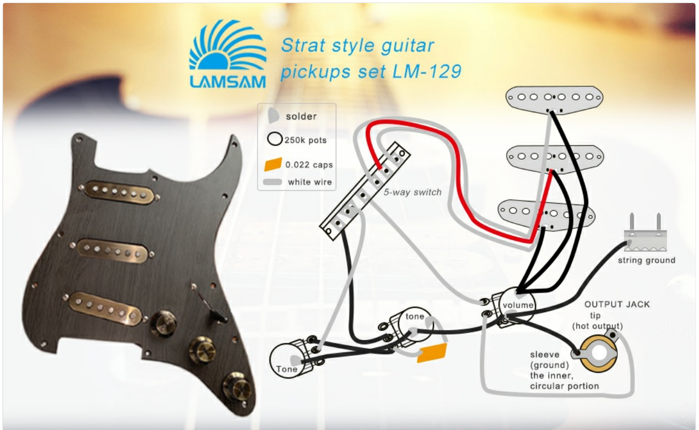
Image: Detailed wiring diagram for the LAMSAM SSS pickup set, including recommended components like 250k pots and 0.022 caps, along with physical dimensions of the pickups.
