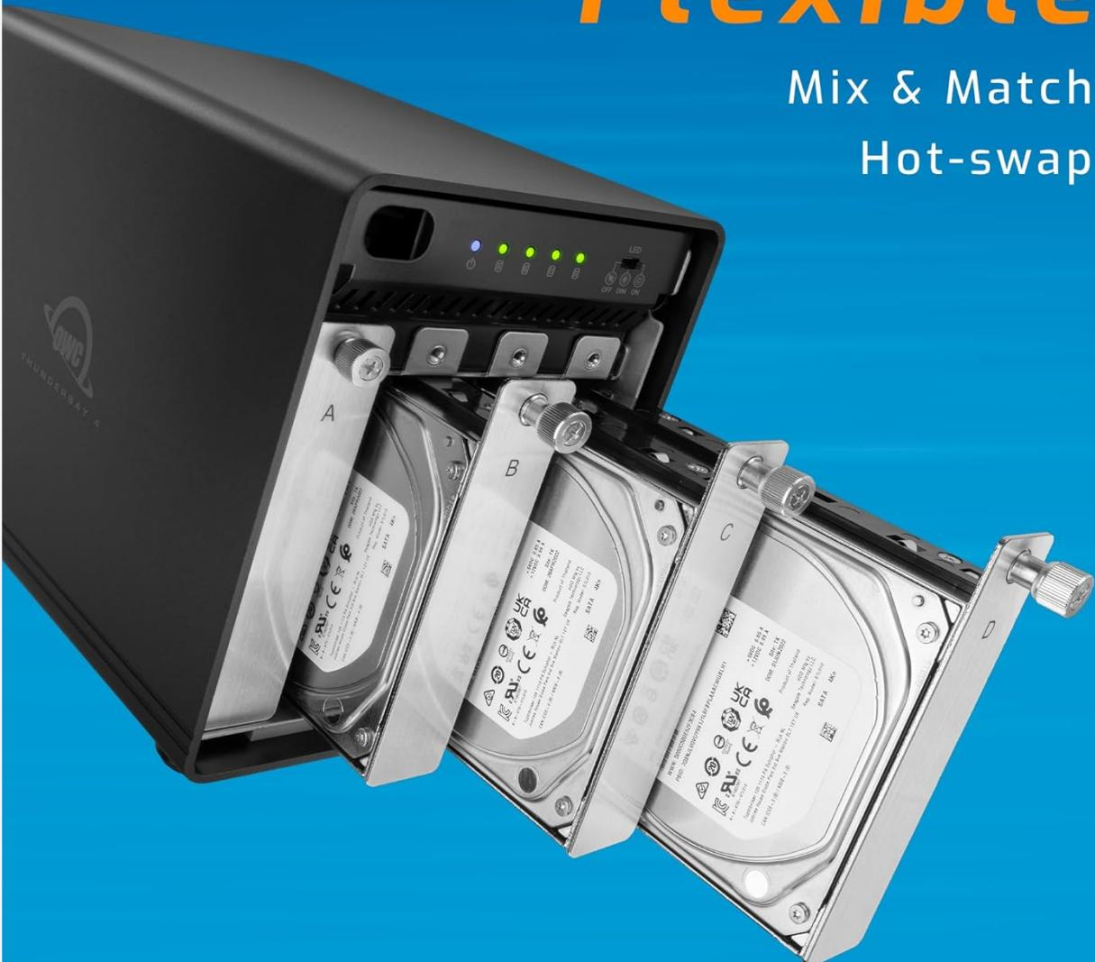
Illustration of drives being inserted into the flexible, hot-swappable bays of the ThunderBay 4.
