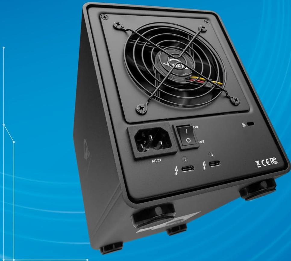
Rear view of the ThunderBay 4, highlighting the built-in power supply and Thunderbolt 3 ports for easy connection.
