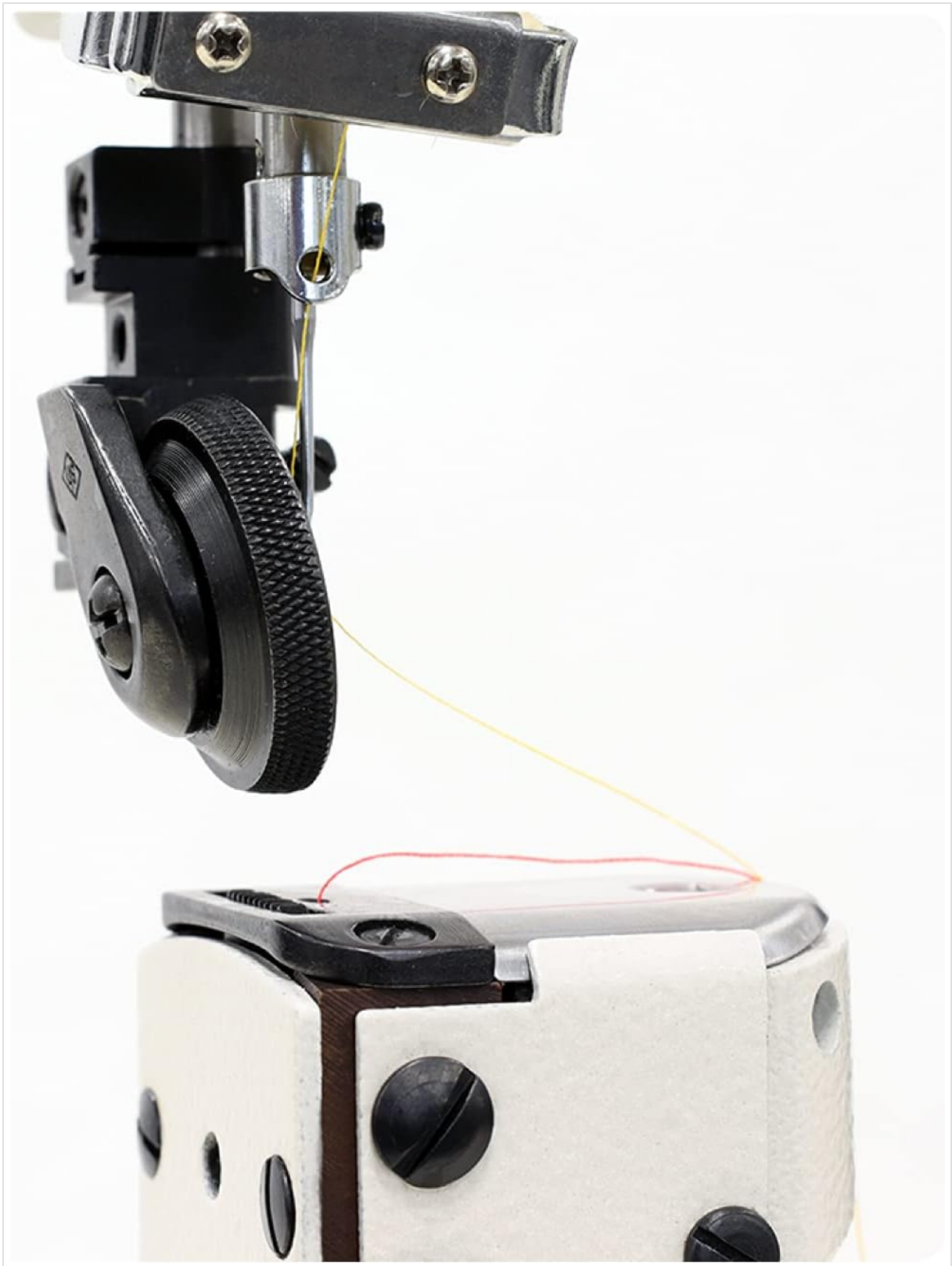
Figure 1: Roller foot and threading path. The yellow thread is guided through the machine's components towards the needle.
