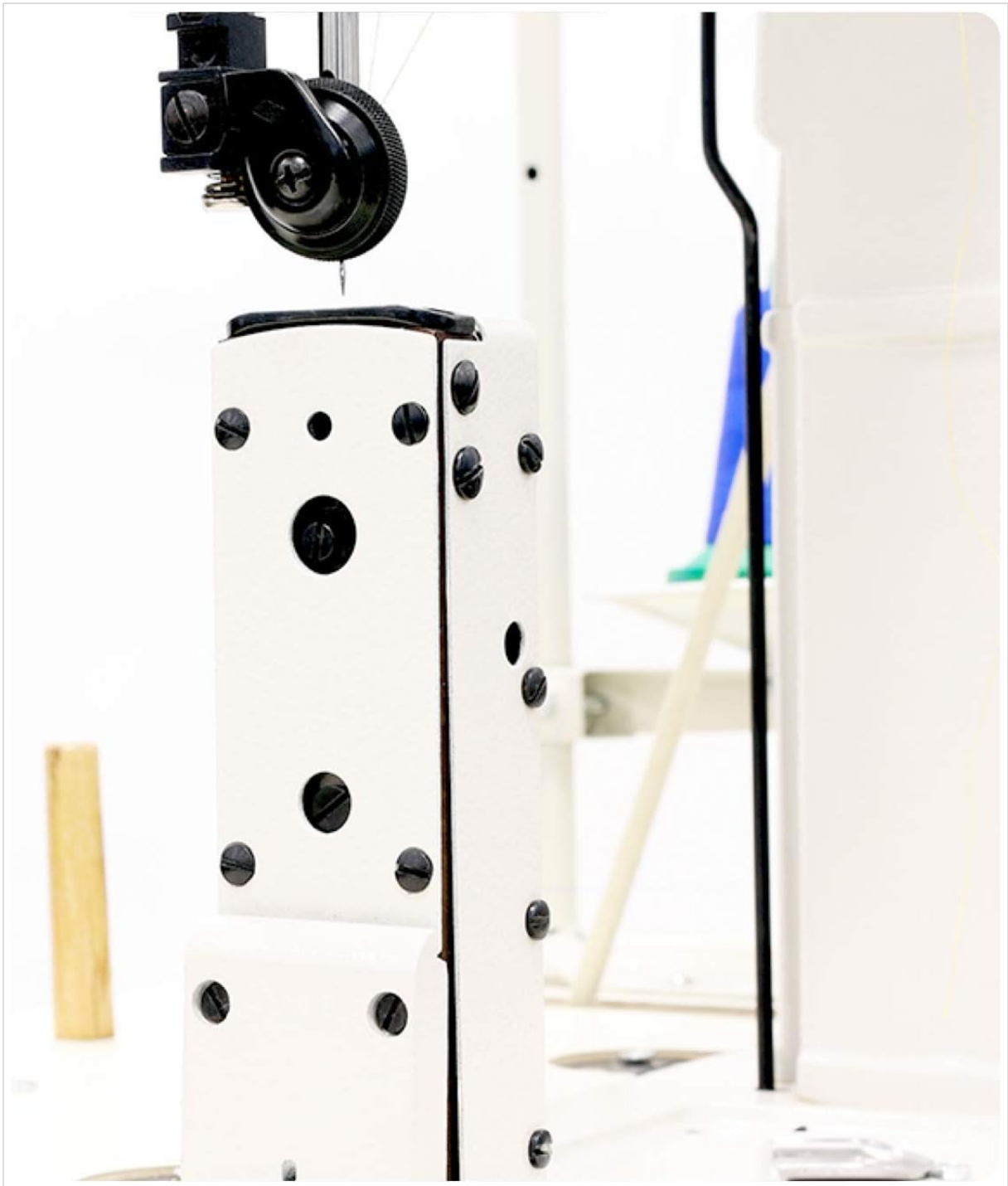
Figure 2: Post-bed design with needle and presser foot area. The elevated post bed facilitates sewing on three-dimensional items.
