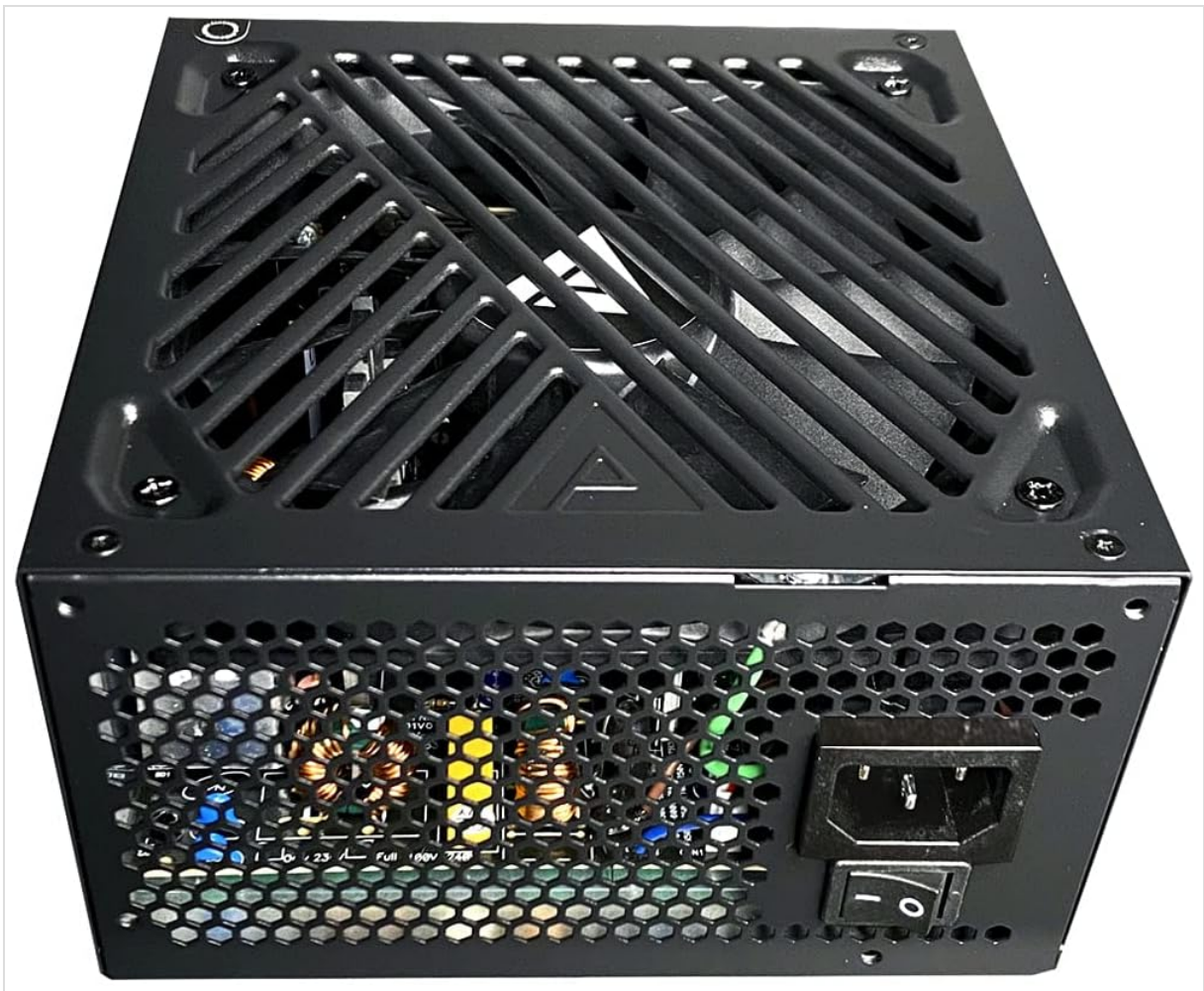
Figure 5: Power Supply Rear Panel with AC Input and Switch
