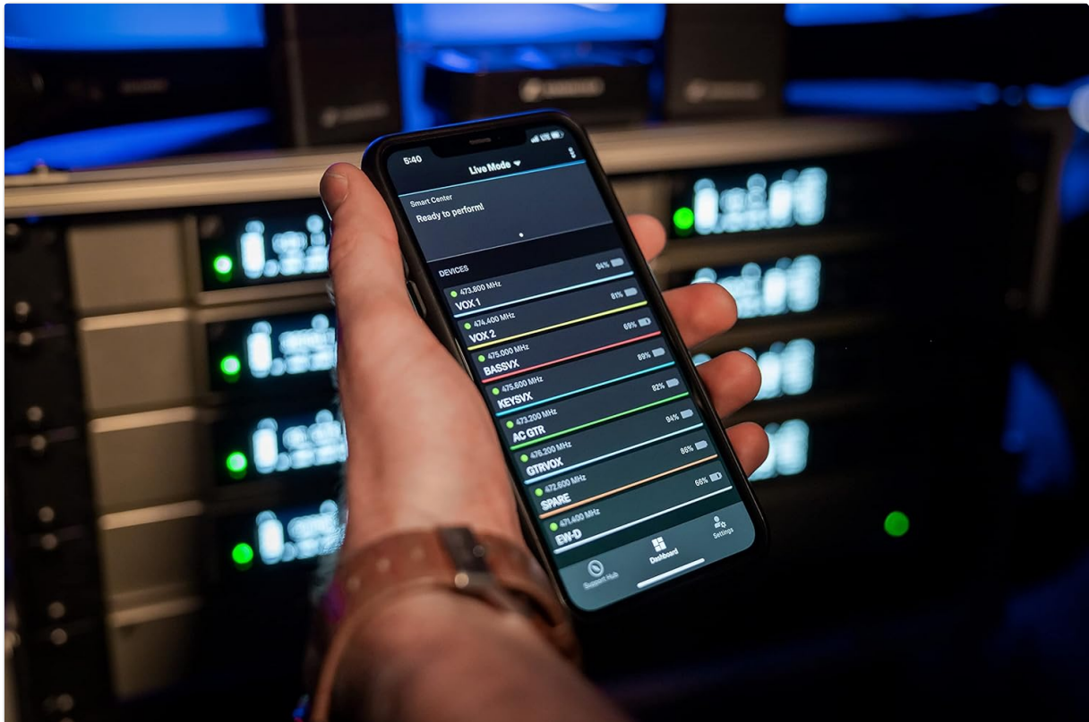
Image 4.2.1: A smartphone displaying the Sennheiser Smart Assist App, which allows for easy management and monitoring of the wireless system.
