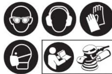
Figure 6: Universal safety icons indicating the necessity of eye protection, hearing protection, gloves, a dust mask, and reading the instruction manual.
