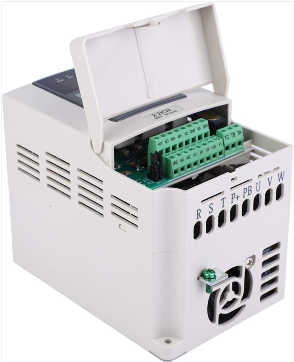
Figure 5.1: Top view of the VFD with the terminal cover open, revealing the input (R, S, T), output (U, V, W), braking (P+, PB), and control terminals for wiring connections.
