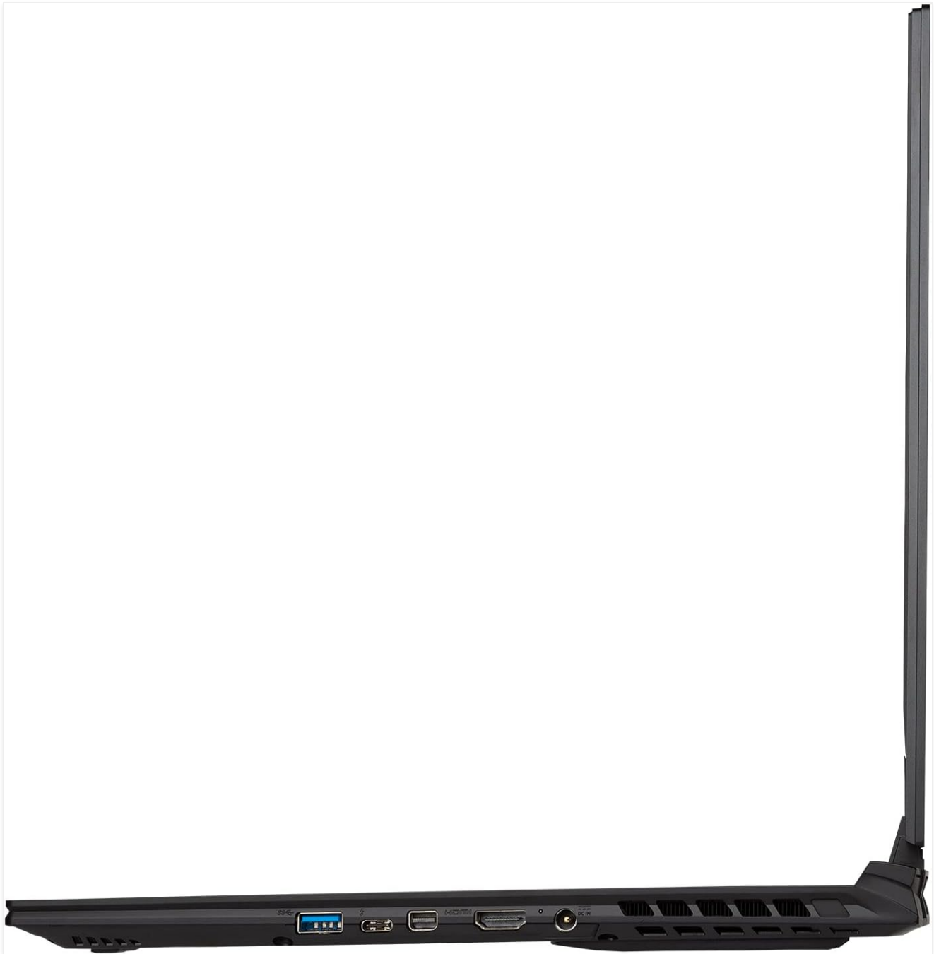
Figure 3: Right Side Ports. This image displays the right side of the laptop, showing ports such as USB 3.0, Thunderbolt 4 (Type-C), Mini DisplayPort, HDMI, and the DC-in power port.
