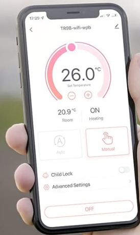
Figure 6: A smartphone screen showing the Tuya Smart app interface, used for remote control of the thermostat.
