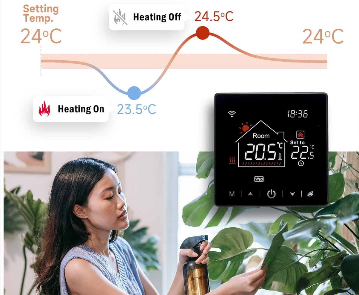
Figure 8: Diagram illustrating temperature hysteresis, where heating activates and deactivates around the set temperature with a 0.5°C differential.
