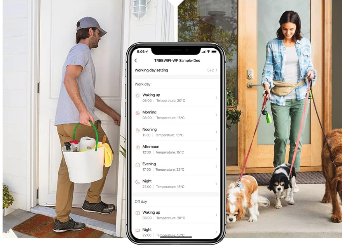
Figure 5: Example of a weekly programmable schedule, showing different temperature settings for various times of the day.
