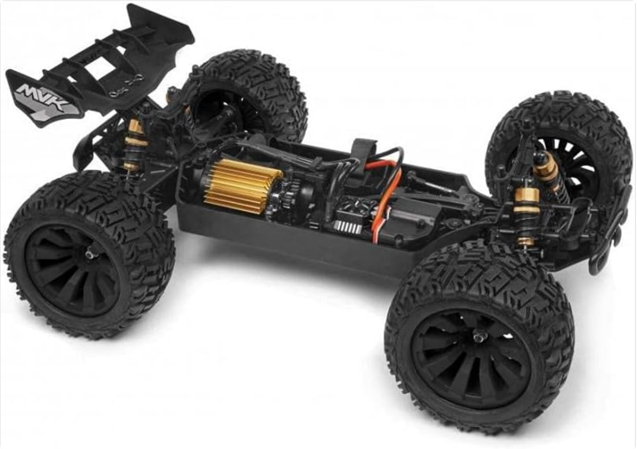
Figure 4.1: Chassis layout of the Quantum+ XT Flux, highlighting the placement of the motor and electronic components.
