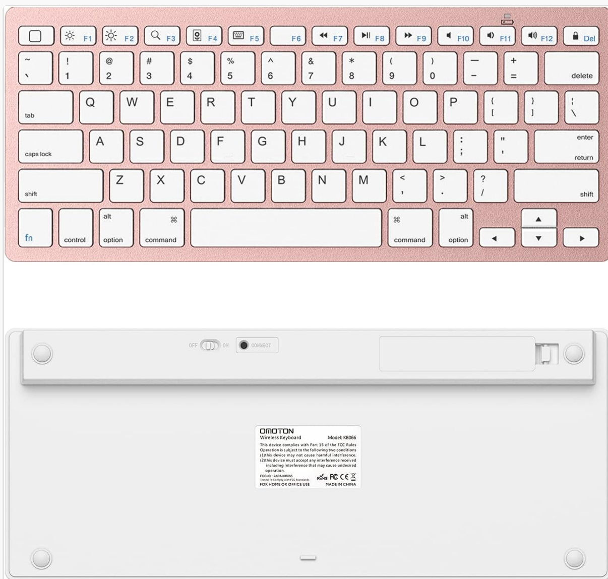
Image 4.1: Top and bottom view of the keyboard, highlighting the power switch, connection button, and battery slot.
