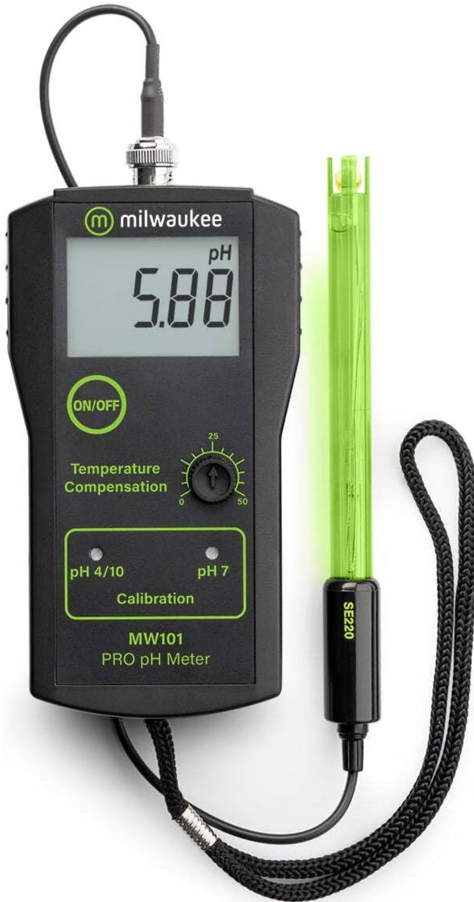
Figure 3.1: Generic MW101 PRO pH Meter with connected electrode. The meter displays pH readings and has controls for temperature compensation and calibration.
