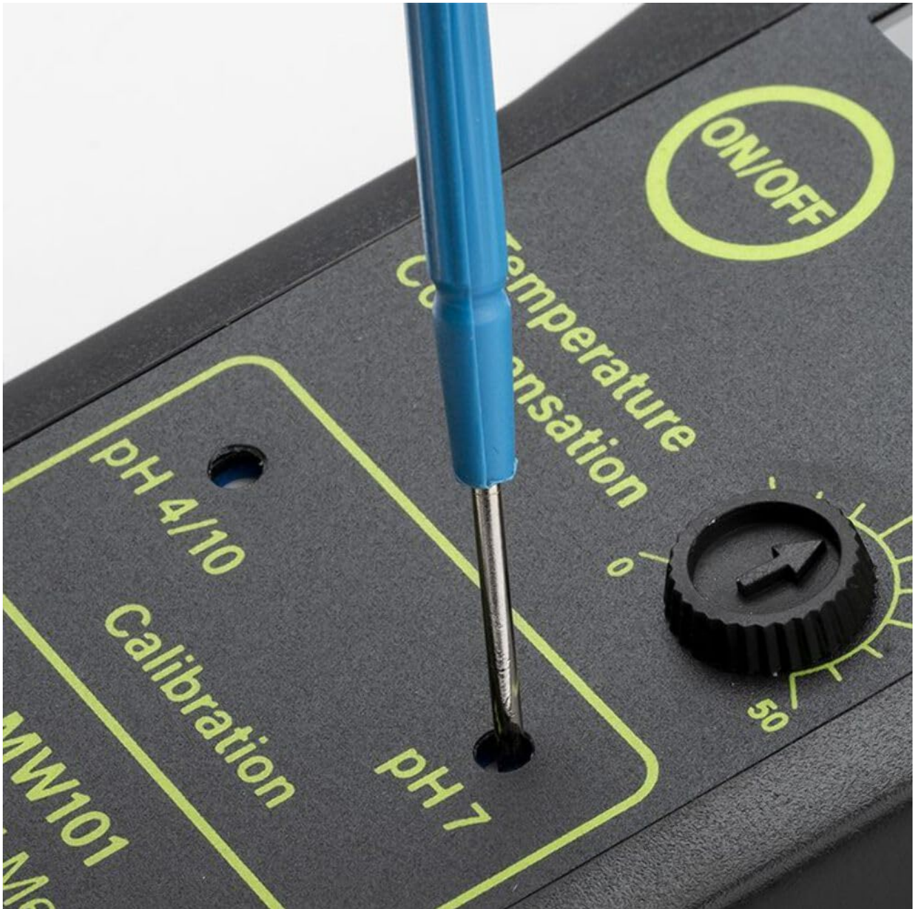
Figure 5.1: Close-up view of the calibration trimmers for pH 4/10 and pH 7, and the temperature compensation dial on the MW101 PRO pH Meter. A screwdriver is used to adjust the trimmers.
