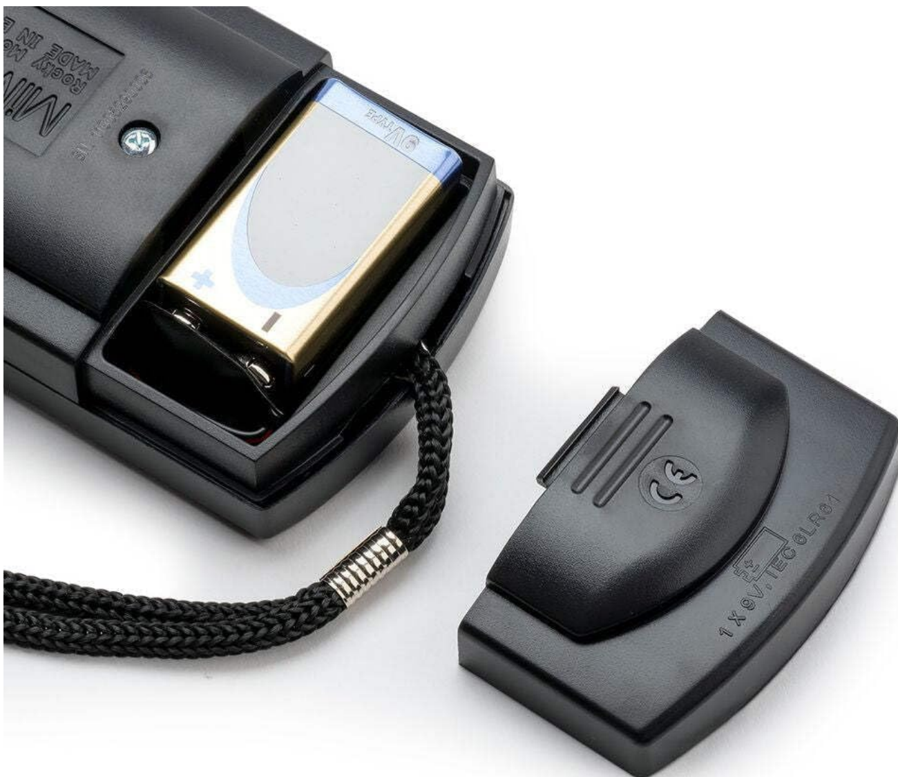
Figure 4.1: Illustration of inserting the 9V battery into the battery compartment of the MW101 PRO pH Meter.
