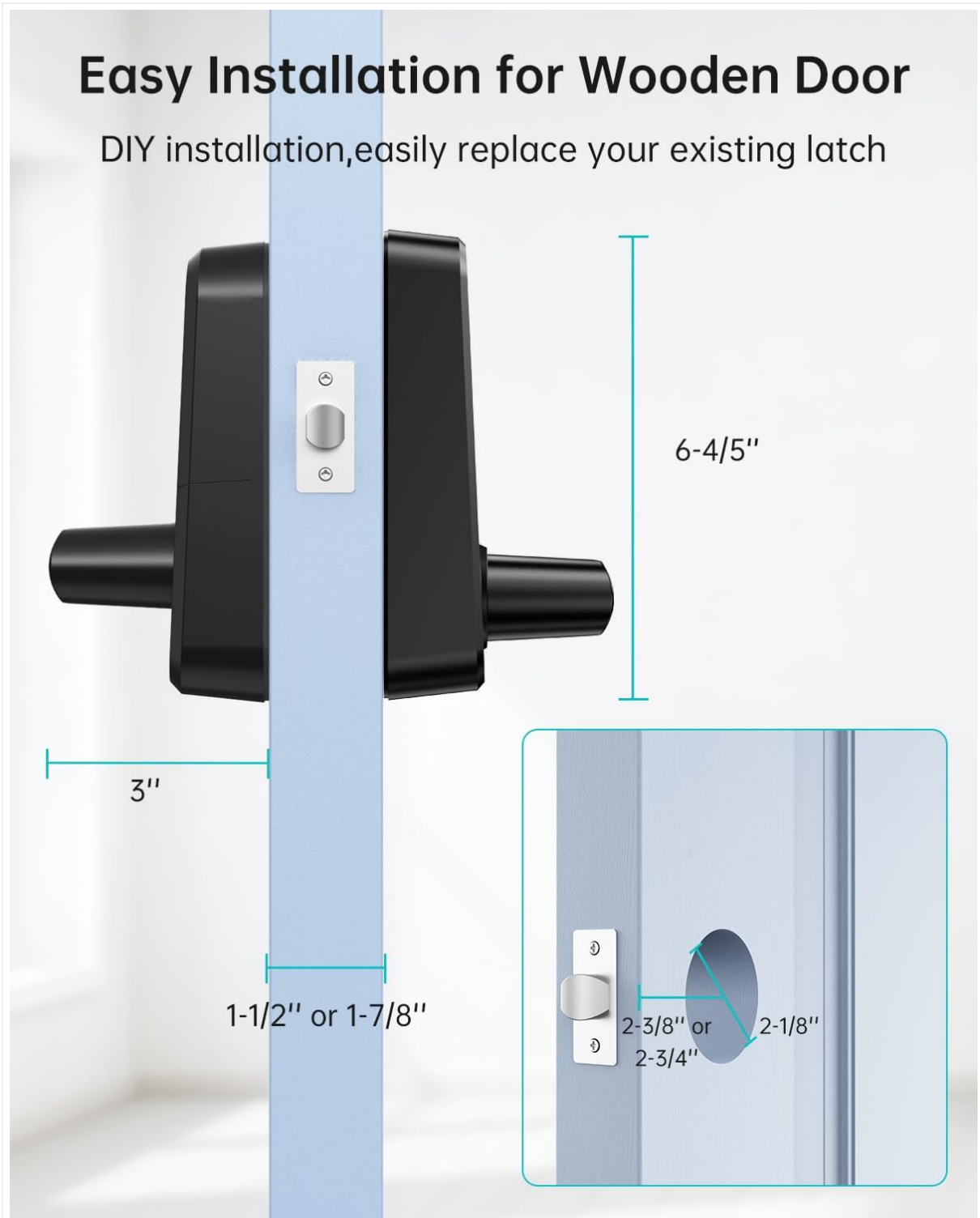
Figure 4.1: Door preparation and dimensions.
