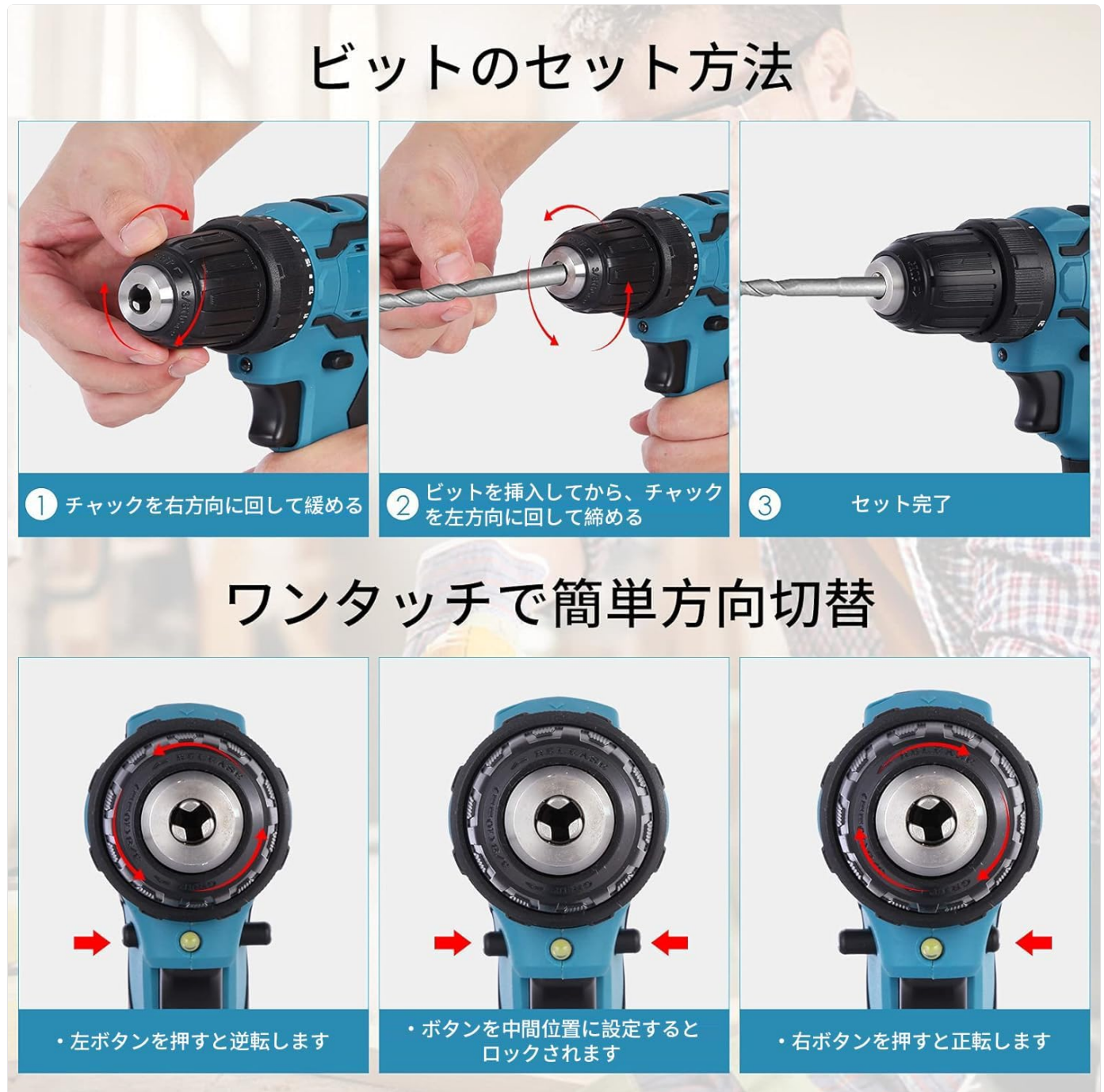
Figure 4.2: Bit Installation and Direction Change. This image illustrates how to loosen and tighten the chuck for bit installation, and how to use the forward/reverse switch.
