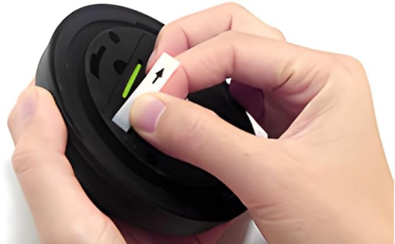
2. Remove the insulation tab
