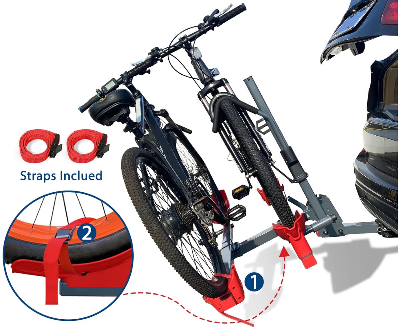
Figure 5.1: Securely loading bikes using wheel cradles and straps.
