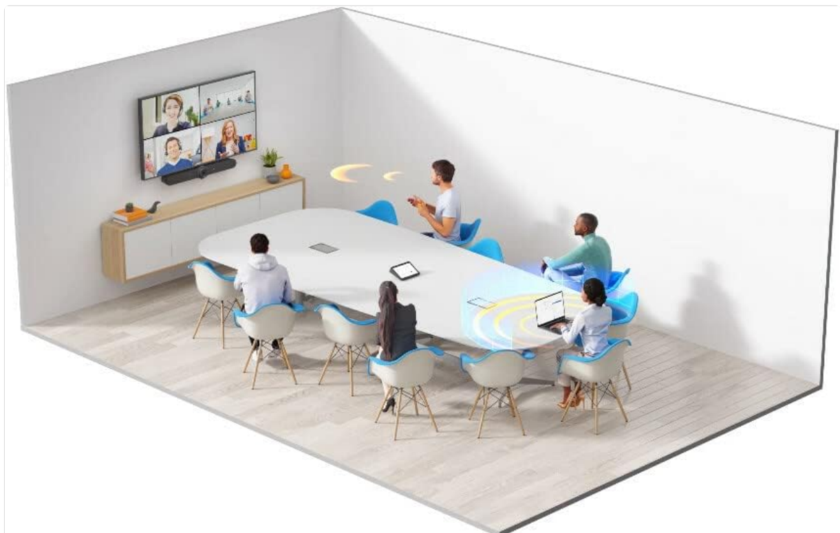
Figure 4.2: Illustration of Rally Bar's AI framing and microphone coverage in a meeting space.
