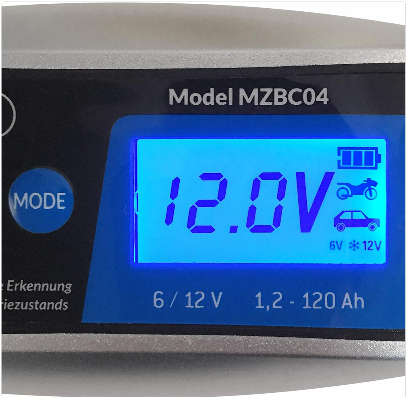
Image: A close-up view of the Monzana MZBC04's LCD display, showing a reading of 12.0V, indicating the current battery voltage during operation.
