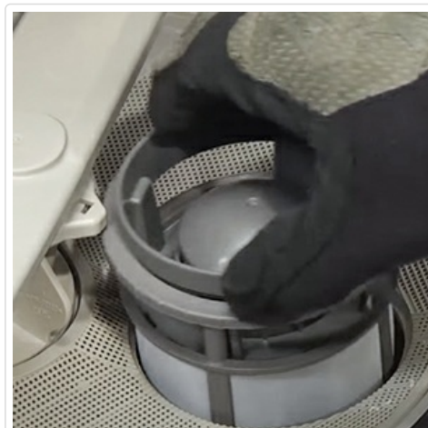
Image: A gloved hand demonstrating the twisting motion required to unlock and remove the dishwasher filter from its housing.
