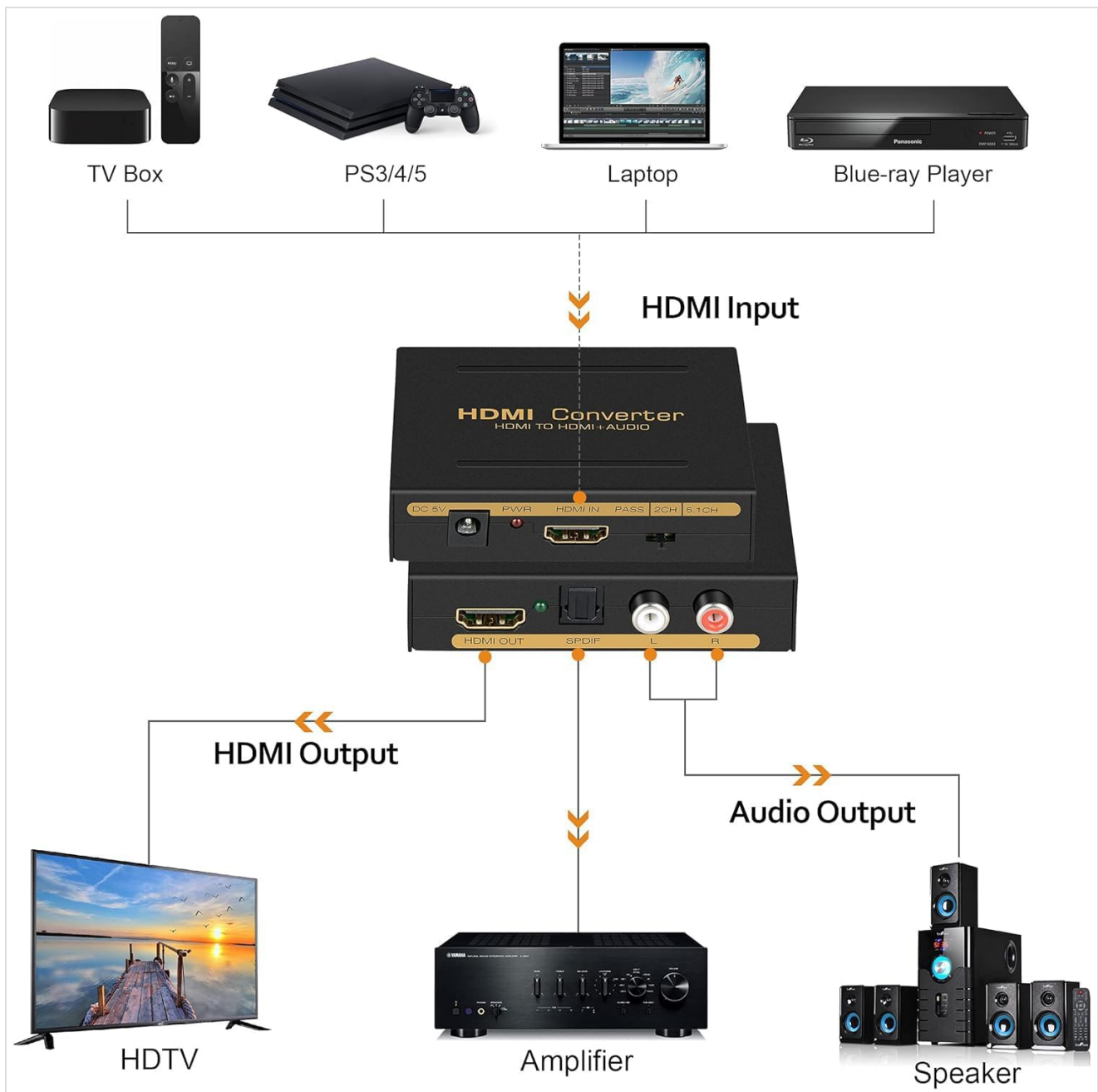
Image 5.1: Typical connection diagram for the HDMI Audio Extractor Converter.
