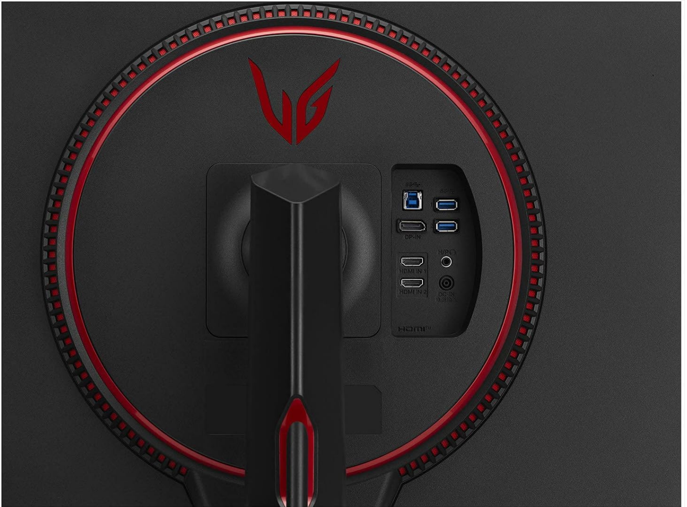
Close-up of the monitor's connectivity ports: DisplayPort, HDMI, USB upstream, and USB downstream.
