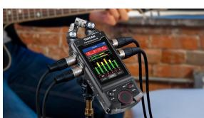
The Portacapture X8 in an active recording session, connected to external microphones via its XLR/TRS inputs,
