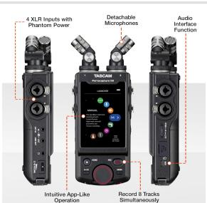
Front view of the Portacapture X8 highlighting its 4 XLR inputs, detachable microphones, intuitive app-like operation, and audio interface function.
