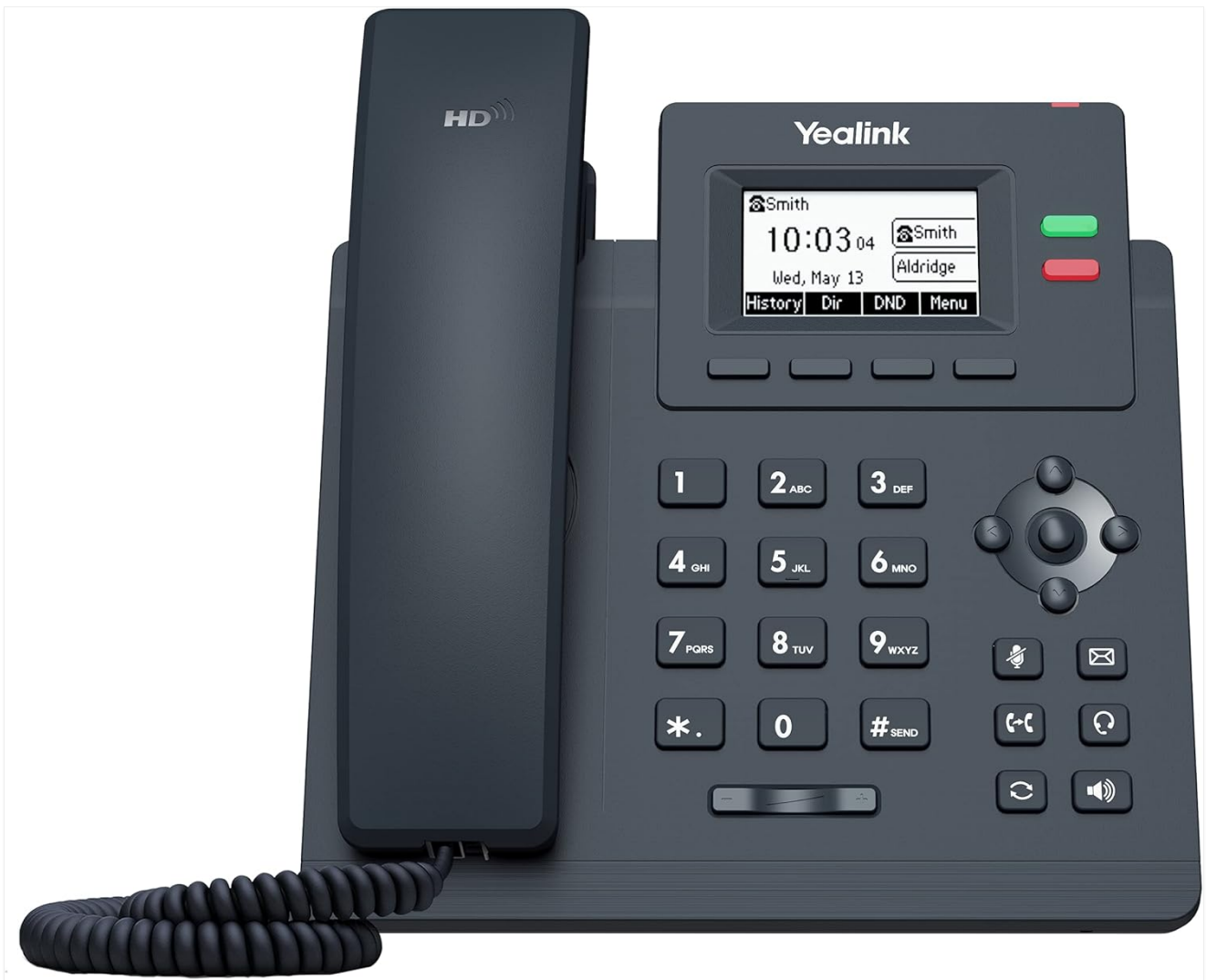
This image displays the front of the Yealink T31G IP Phone, showing the main display, keypad, navigation cluster, and function buttons. The handset is cradled on the left side, and the phone is presented in a dark gray finish.
