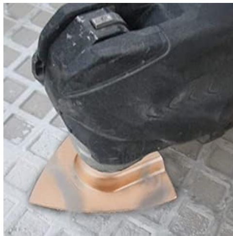
A close-up image showing a triangular carbide blade actively grinding away tile grout, demonstrating its effectiveness in surface preparation.
