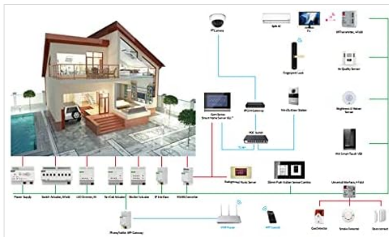
Figure 2: Typical KNX System Diagram
