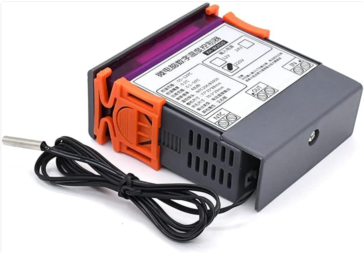
Figure 5.1: Wiring terminals for the Q-BAIHE W2020 thermostat. The 'IN' terminals are for power input (220V AC), 'OUT' terminals are for connecting the heating/cooling load, and 'NTC' terminals are for the temperature sensor.
