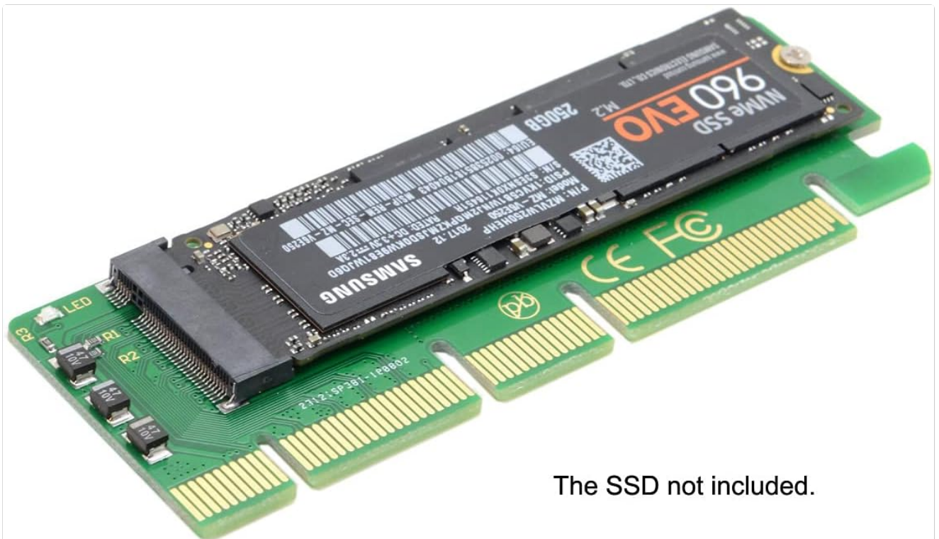
Image: An M.2 NVMe SSD correctly installed and secured onto the NFHK PCI-E adapter.
