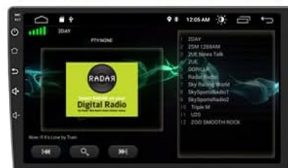
Figure 5.5: Overview of Features. This image presents a comprehensive overview of the car radio's functionalities, including its Android operating system, Bluetooth for music and hands-free calls, FM/RDS radio, compatibility with steering wheel controls, split-screen mode, MirrorLink for smartphone mirroring, and optional support for DAB+, rearview camera, and front camera.
