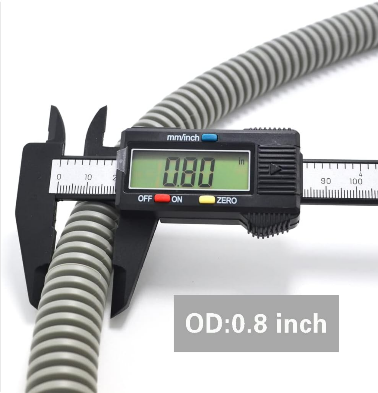
Image 6.1: Measurement of the hose's outer diameter, indicating 0.8 inches.
