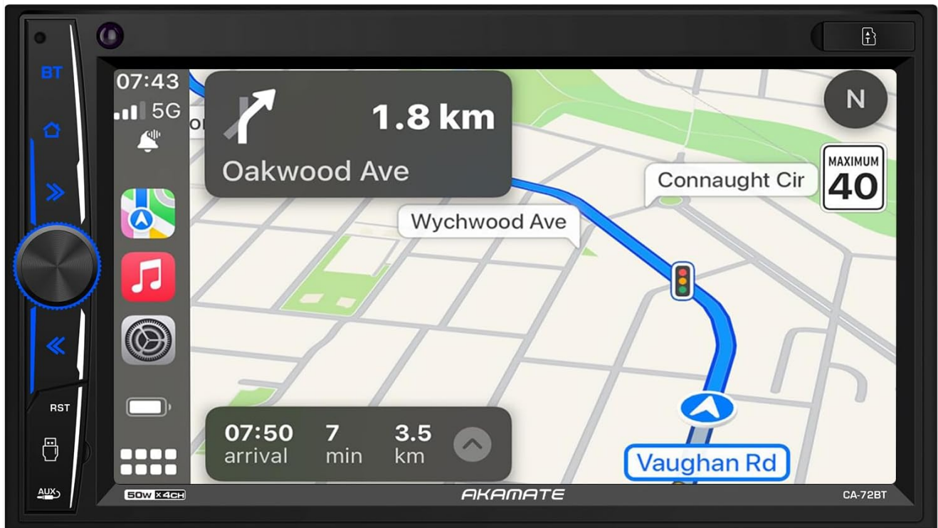
Image 5.3: Mirror Link feature displaying a phone's navigation screen on the car stereo. This image shows the stereo screen mirroring a navigation application from a connected smartphone.
