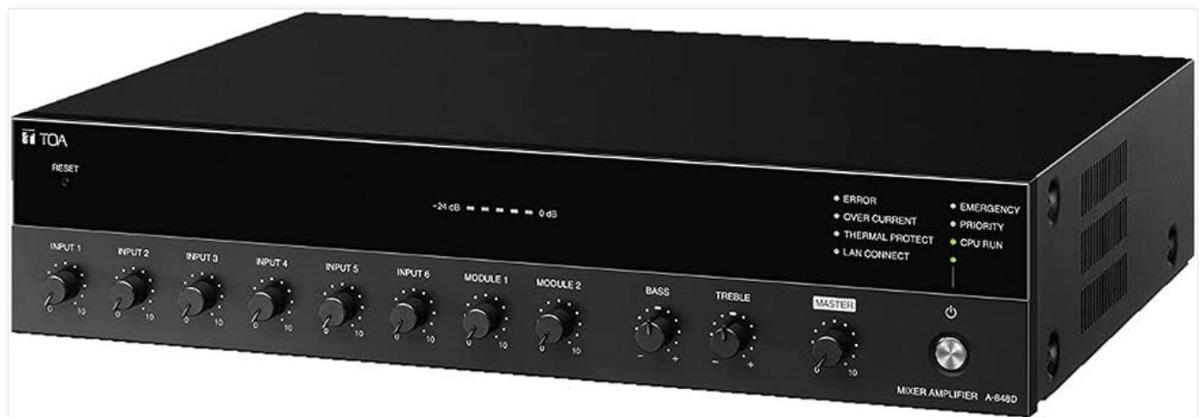
Figure 4.1: Front Panel of the TOA A-848D. This image displays the front of the amplifier, featuring six input level controls, two module level controls, Bass and Treble tone controls, a Master volume knob, and a power button. An LED display shows output levels, and status indicators for Error, Over Current, Thermal Protect, LAN Connect, Emergency, Priority, and CPU Run are visible.
