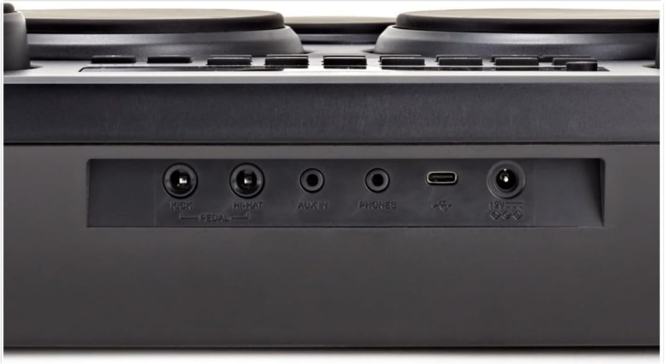
Image: Rear panel of the DD80 unit, illustrating the various input and output ports, including those for the kick and hi-hat pedals.
