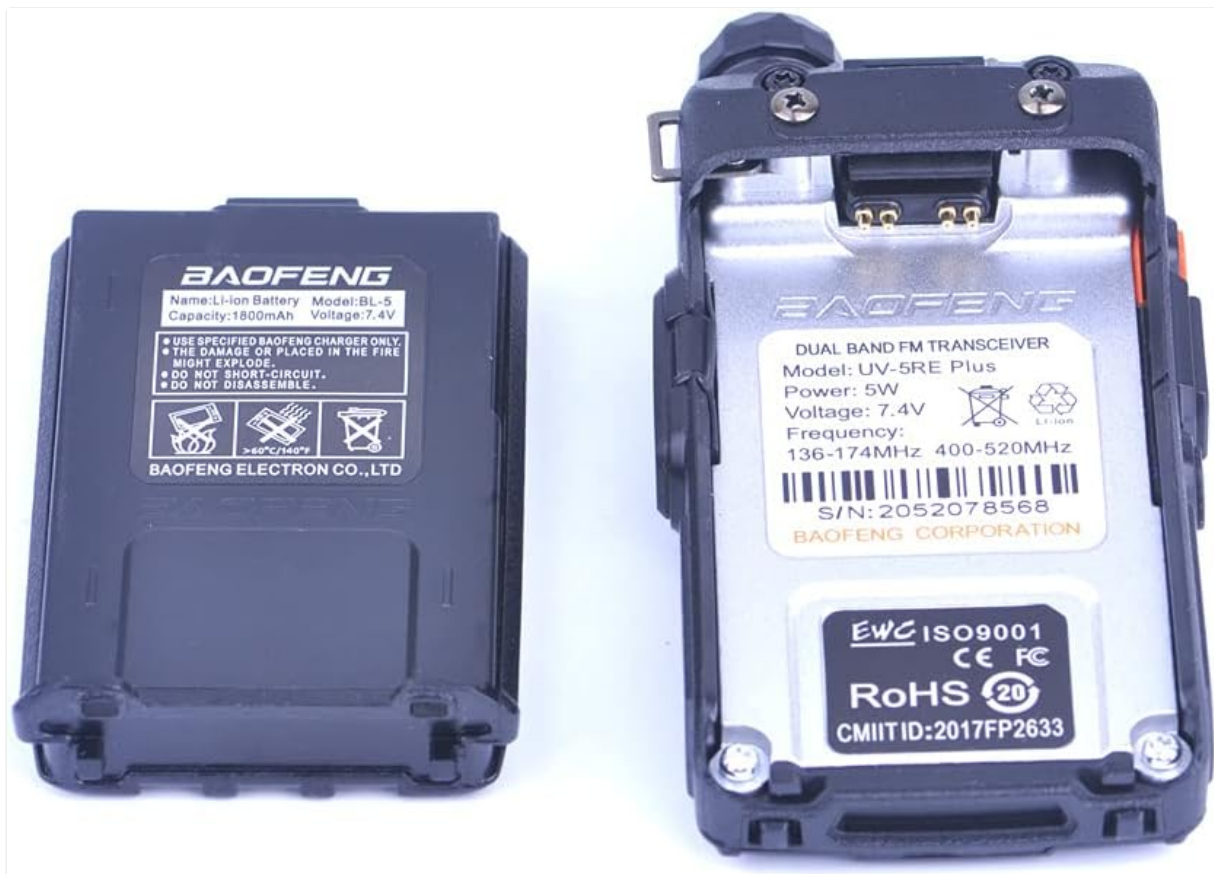
Image: The NSKI UV-5RE Plus radio with its battery pack detached, showing the battery contacts on both the radio and the battery. This illustrates how the battery connects to the radio.
